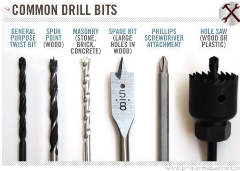
It's recommended only to use general purpose, spur point, and screwdriver bits with manual drills. Other bits require more torque to operate.
